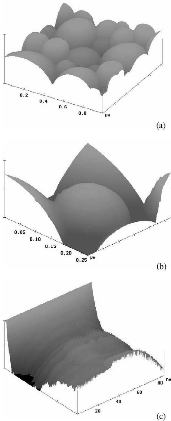
Fig. 3. AFM images of nanoparticles prepared with TPGS as emulsifier: (a) multi-particles; (b) single particle; (c) zoom-in of the nanoparticle surface.
