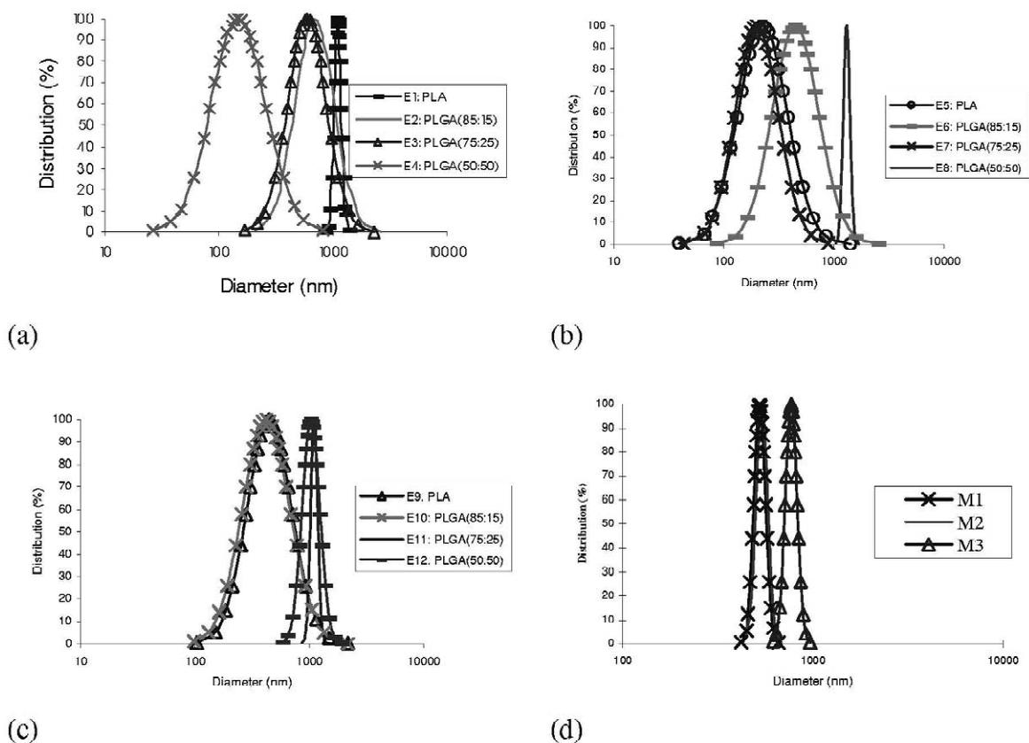
Fig. 4. Size distribution of produced nanoparticles under various experiment parameters: (a) TPGS as emulsifier with high concentration (0.06%); (b) TPGS as emulsifier with medium concentration (0.03%); (c) TPGS as emulsifier with low concentration (0.015%); (d) TPGS as matrix blended with PLGA with no other emulsifier (ratio for PLGA-TPGS: M1 (2:1), M2 (1:1), M3 (1:2)). The horizontal axis is plotted on log-normal scale.
