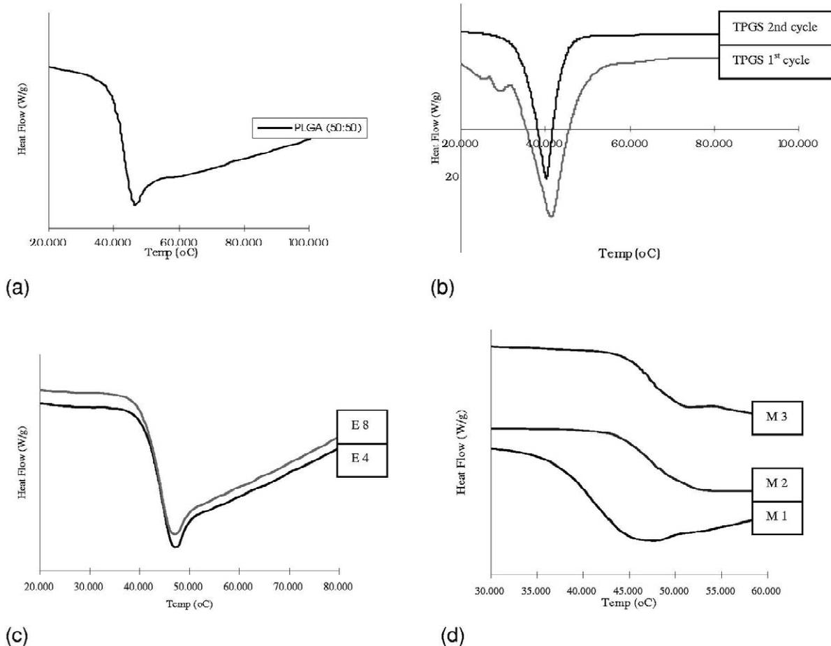
Fig. 5. DSC thermogram of second heating cycle of fabricated nanoparticles and related material: (a) pure PLGA (50:50); (b) pure TPGS; (c) PLGA nanoparticles with TPGS as emulsifier; (d) nanoparticles with blended mixture of PLGA and TPGS as matrix.
