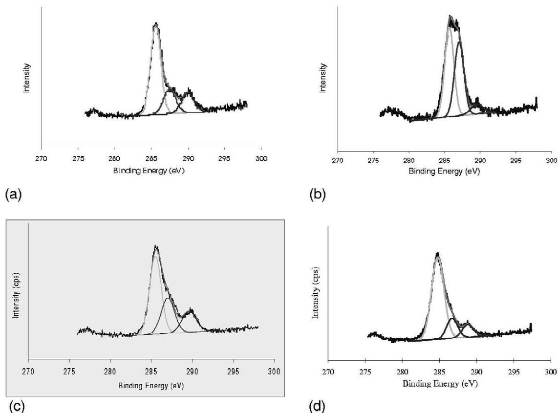
Fig. 6. Surface chemistry analysis of C1s with X-ray photoelectron spectroscopy: (a) PLGA (50:50); (b) vitamin E TPGS; (c) PLGA (50:50) nanoparticles using TPGS as emulsifier; and (d) PLGA-TPGS (1:1) nanoparticles.
